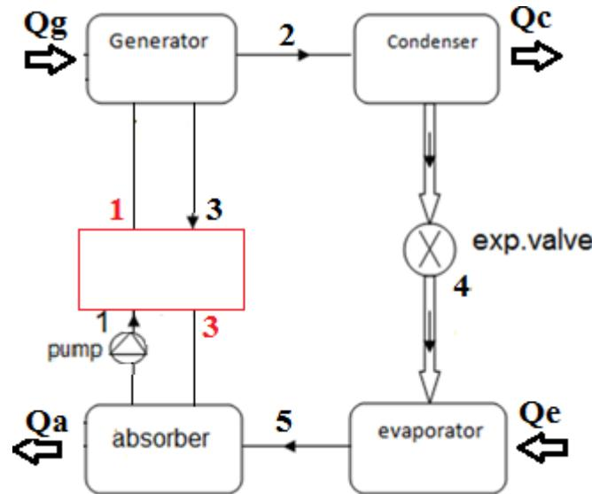
$P_g = P_c = \text{high pressure at } T_{sat} = 38^\circ\text{C}$
